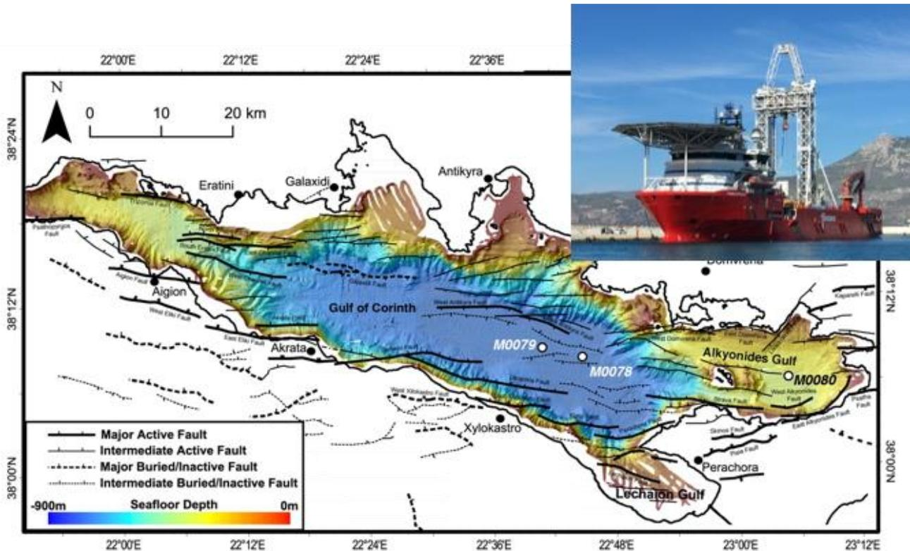
**Figure 1. Fault and bathymetry map (after Nixon et al., 2016) of the Gulf of Corinth and Corinth Rift, showing the locations of the 3 IODP boreholes (M0078-M0080). Inset shows the Fugro Synergy geotechnical vessel that performed the drilling.**
