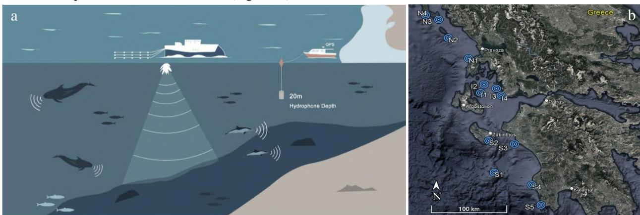
Figure 1. (a) The acoustic monitoring set-up and (b) the monitoring stations (blue circles).
