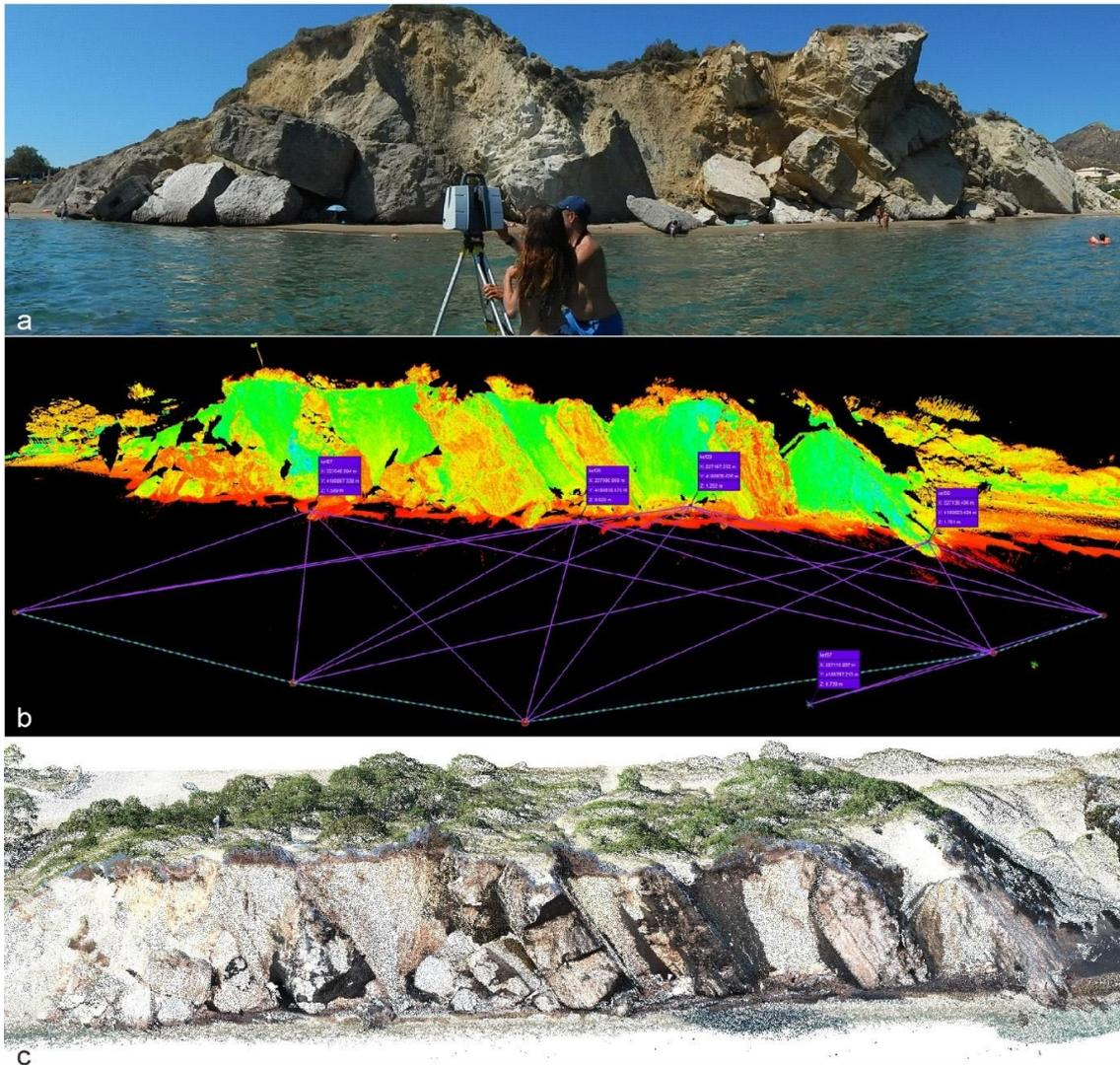
**Figure 1.** Using the TLS for the point-cloud data acquisition of the steep slope (a). Construction of the 3D model after the alignment of the six datasets and registration with the ground control targets (b). Combination of the two datasets of pointclouds (from TLS and UAS).
