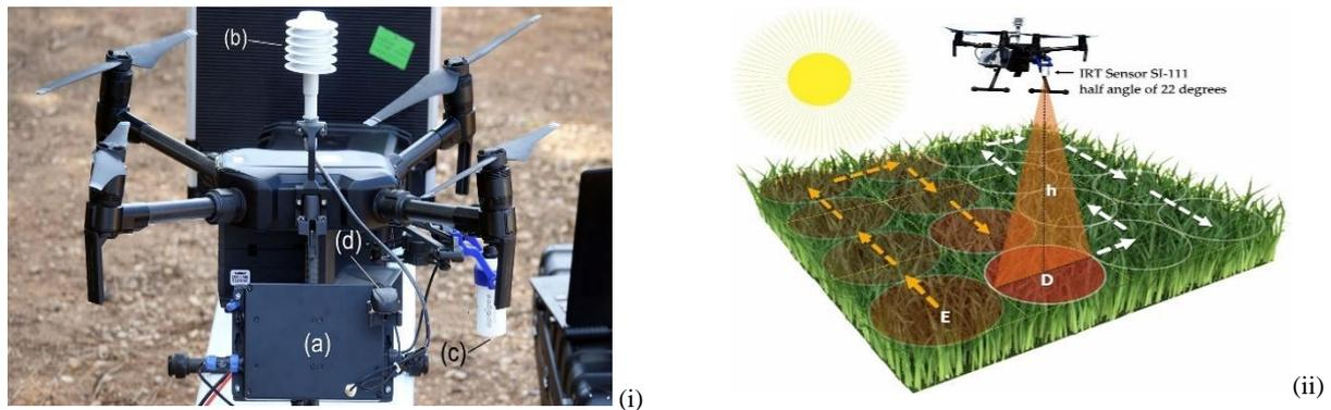
**Figure 1. (i) (a) Data logger Stylitis-12; (b) thermo-hygrometer sensor; (c) IR-TH infrared sensor; (d) GPS sensor, (ii) Graphic illustration of the measurement process with an infrared radiometer adapted to a UAV over dense cultivation foliage under a clear sky. The flight height depends on the sensor type and the characteristics of the crop.**
