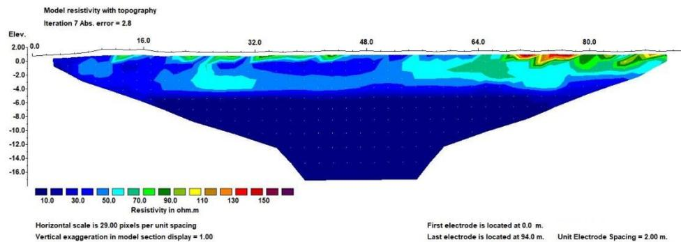
Figure 2. Electrical resistivity tomography at Kotichi site.
