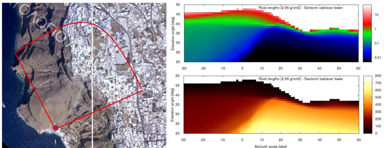
**Fig.1. Left: Proposed position of the muographic telescope. Right top: simulated muon flux through the Fira fault, Santorini, for various azimuth angles. Right bottom: calculated rock length around the Fira fault for various azimuth angles (G. Nyitrai).**
