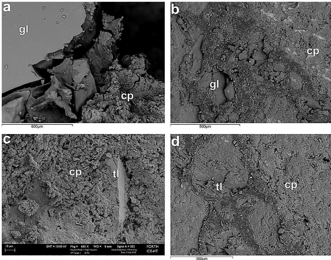
**Figure 1.** Secondary electron images showing microstructures at the interface between cement paste and: (a) beer green glass; (b) beer green glass with quartz primer; (c) waste tile; and, (d) waste tile with quartz primer. gl: glass, cp: cement paste, tl: tile.
