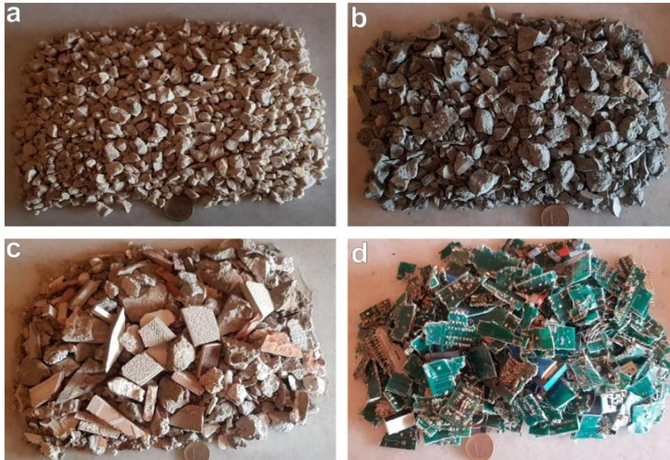
**Figure 2. Representative photos of aggregate components showing: (a) Limestone; (b) Basalt; (c) construction wastes; (d) E-wastes.**
