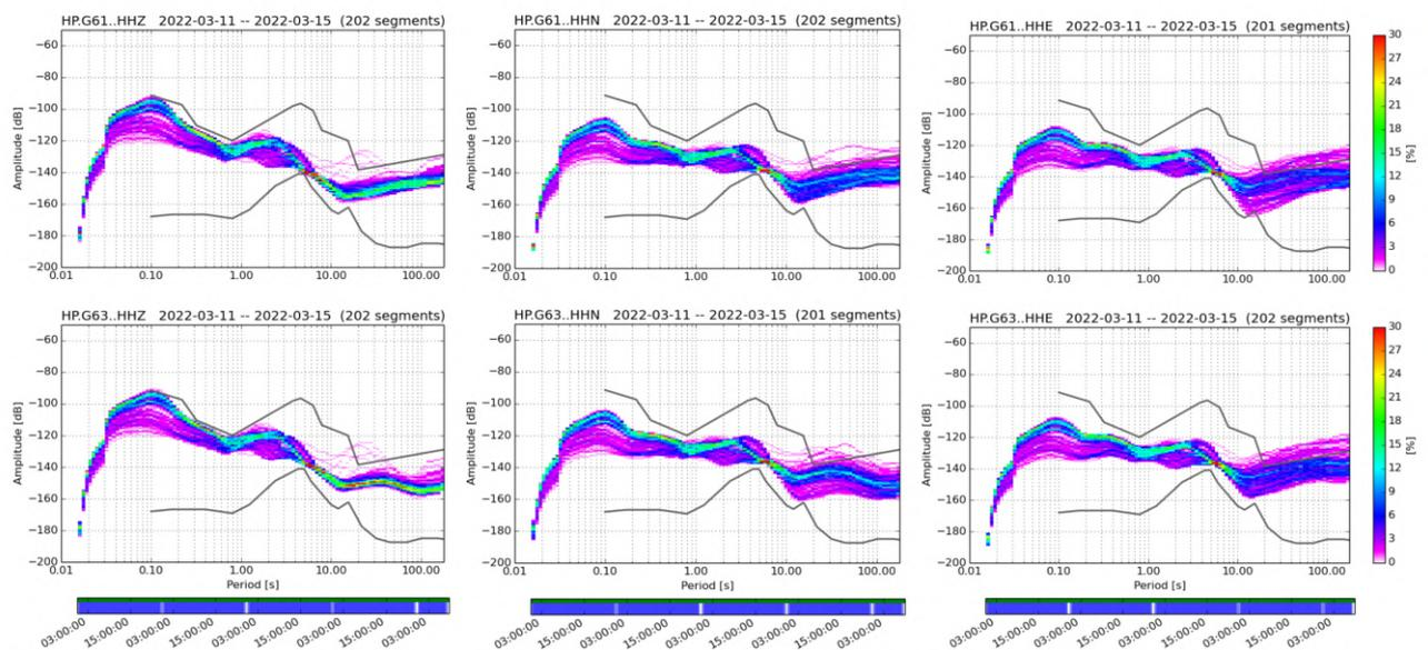
**Figure 2. Power spectral density plots for the reference instrument (top) and the prototype (bottom). From left to right the Z, N and E component is presented.**
