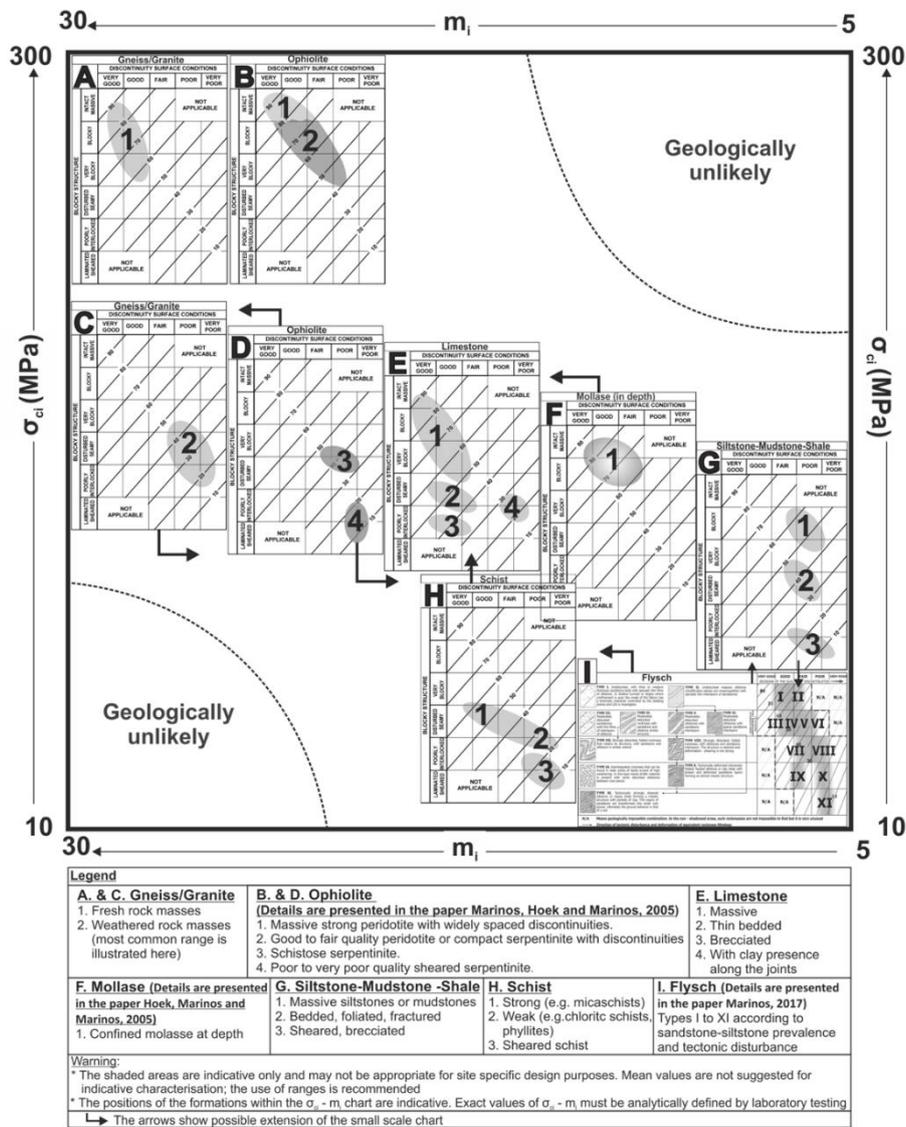
Figure 2. Most common GSI ranges for typical gneisses, granites, ophiolites, limestones, schists, siltstones/mudstones/shales, molassic and flysch formations in conjunction with a range of  $m_i$  and  $\sigma_{ci}$ . (Marinos & Carter, 2018).
