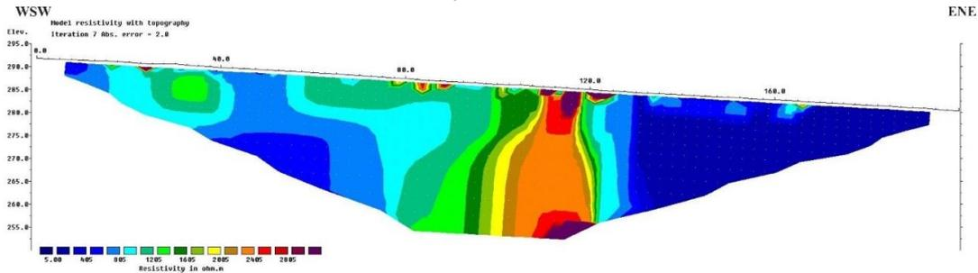
**Figure 2. Electrical Resistivity Tomography**
