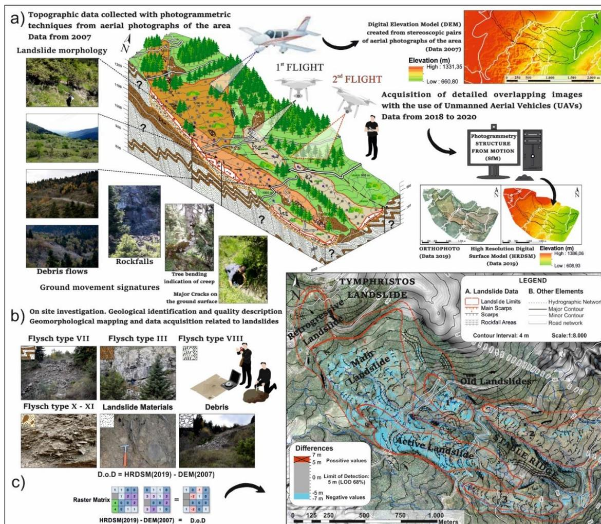
**Figure 1. Schematic representation of operations followed in this research. a) Data acquisition, Geological Model and Digital Surface Models construction. b) Ground investigations. c) Change Detection analysis (DoD construction).**
