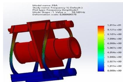
Figure 2. 3D view of the spring-mass system, at the first normal oscillation mode.
