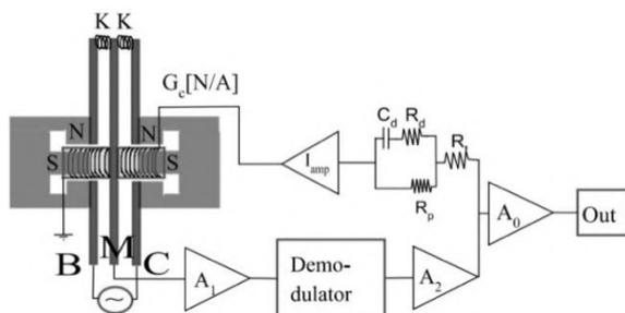
Figure 1. Simplified block diagram of the FBA accelerometer
