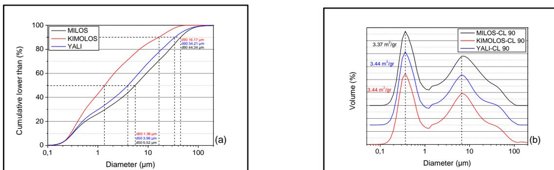
**Figure 1 (a & b).** Particle size distribution of Pozzolanas after the procedure of individual grinding (a) and the resulted granulometry of the Lime-Pozzolana mixtures (b), after co-grinding them with the aid of a micro-Deval apparatus.
