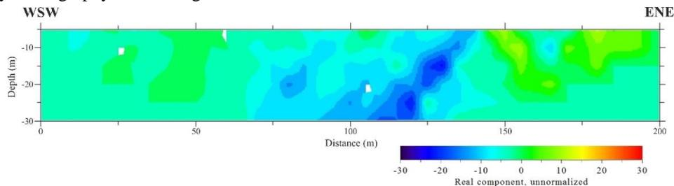
**Figure 3. The Karous-Hjelt pseudo-section for current density distribution**
