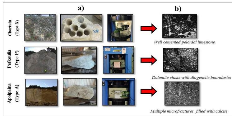
**Figure 1. a) Photographs from the locations of block sampling, typical blocks from each rock type and specimens tested in uniaxial compression; b) Thin sections photomicrographs (PPL) from the three rock types.**
