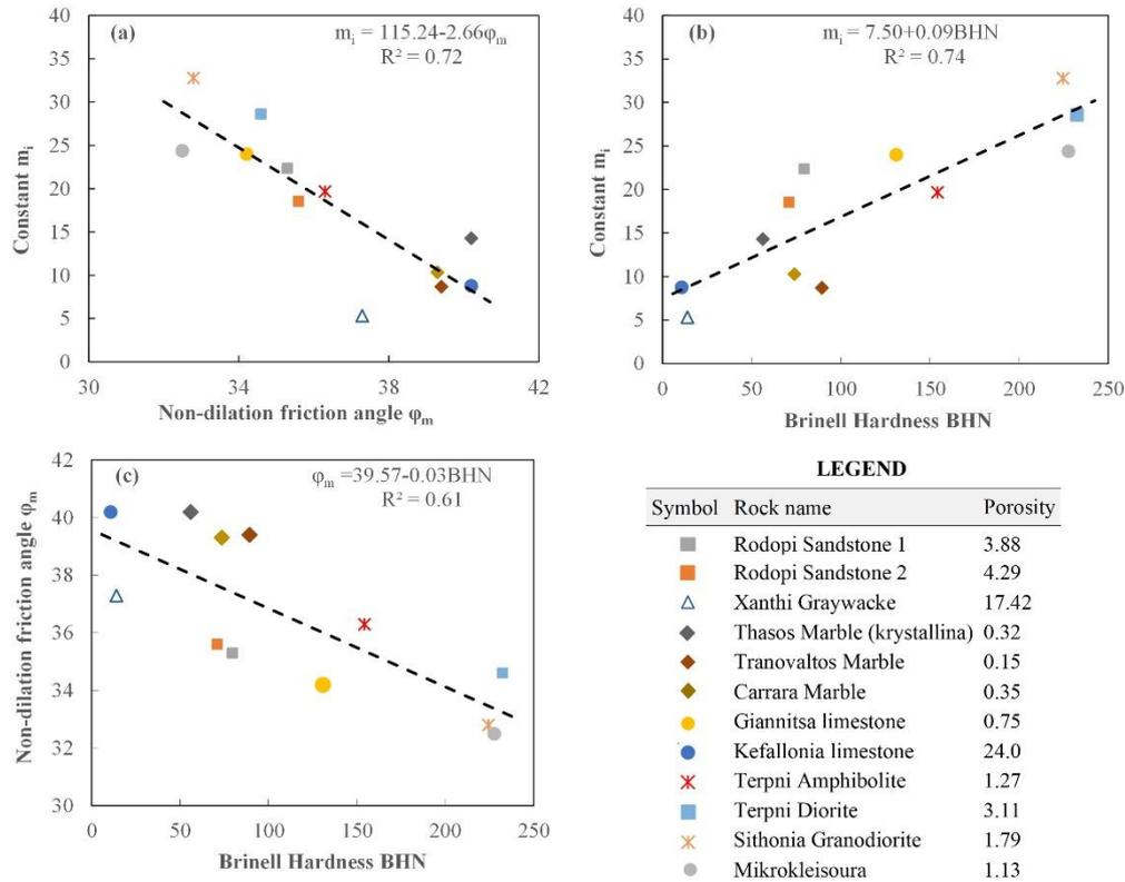
**Figure 1. Graphical representation of the interrelations among non-dilational friction angle of joints  $\phi_m$ , constant  $m_i$  of Hoek-Brown criterion and Brinell Hardness Number BHN. (a) constant  $m_i$  vs. non-dilational friction angle  $\phi_m$ . (b) constant  $m_i$  vs. Brinell Hardness Number BHN. (c) Non-dilational friction angle  $\phi_m$  vs. Brinell Hardness Number BHN.**
