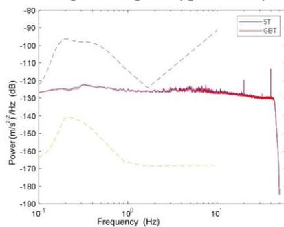
**Figure 3. Total noise PSD diagrams for the proposed accelerometer (GBT) and the reference instrument (5T).**
